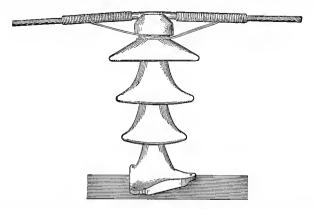
FIG. 34. High tension (60,000 volt) porcelain insulator and iron pin support used on N. Y. State lines of Ontario Power Company.
